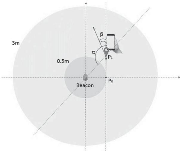
Fig. 4. New user's heading regarding the beacon and general coordinate system after several steps in straight direction
