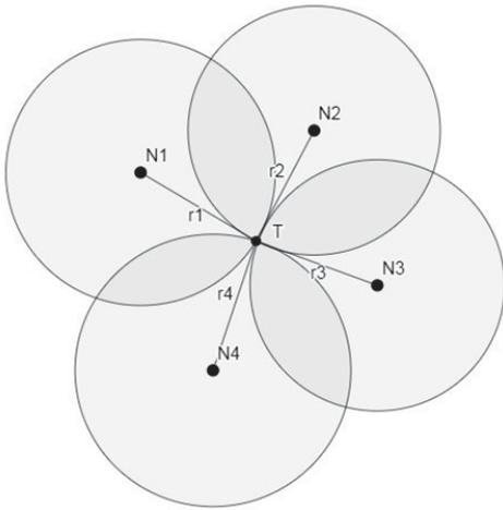
Fig. 1. Target node multilateration by four reference nodes
