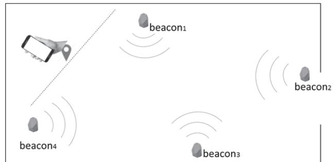
Fig. 5. User heading regarding the beacon after several steps in straight direction
