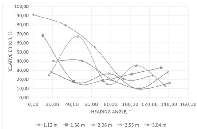
Fig. 6. The dependency between smartphone heading angle and relative error
