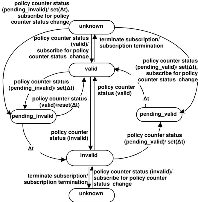
Fig.9. Model of policy counter state as seen by the mobile edge application
