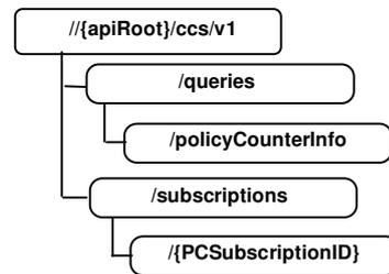
Fig.8 Structure of resources supported by CCS
