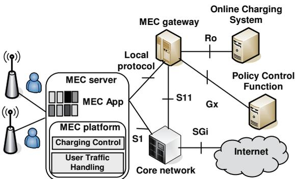
Fig.1 Architecture of MEC system for policy decisions based on subscriber spending limits
