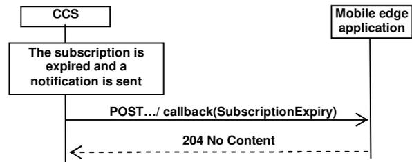
Fig.5 Flow of CCS sending notification on subscription expiry
