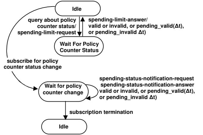
Fig.10. Model, representing the spending limits tracking of given subscriber, supported by the CCS
