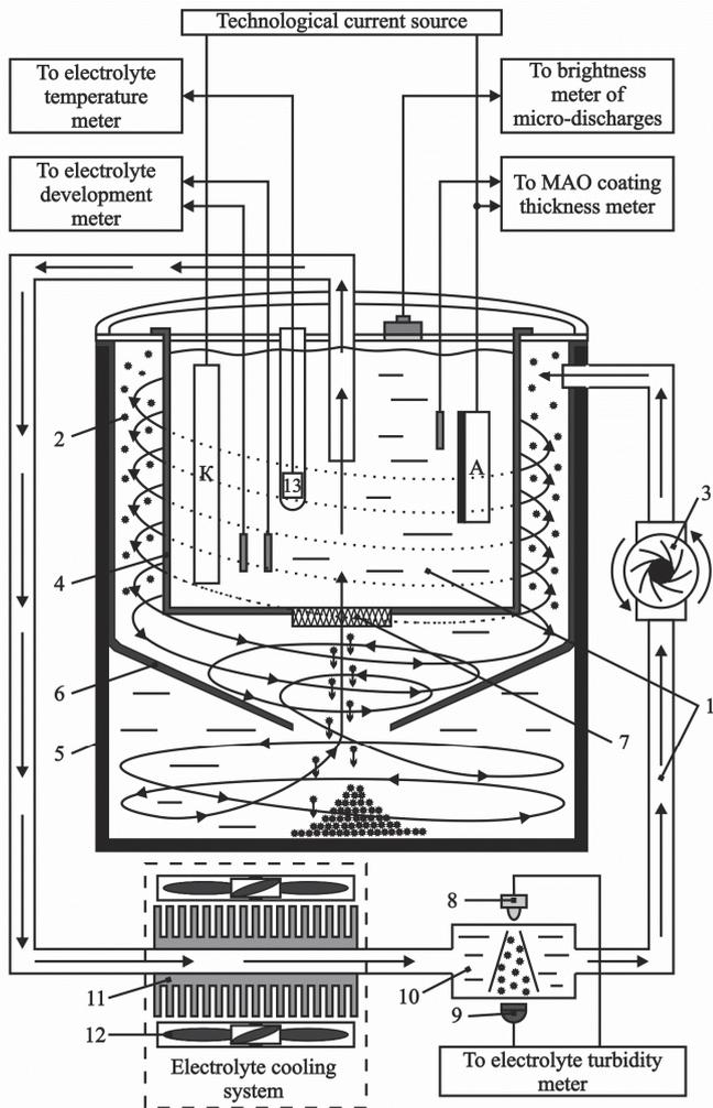
Fig. 5. Construction of the galvanic cell: 1 – electrolyte, 2 – sludge particle, 3 – pump, 4 – electroplating bath, 5 – housing, 6 – cone, 7 – filter, 8 – light emitting diode, 9 – photodetector, 10 – cell, 11 – radiator, 12 – fan, 13 – temperature sensor
