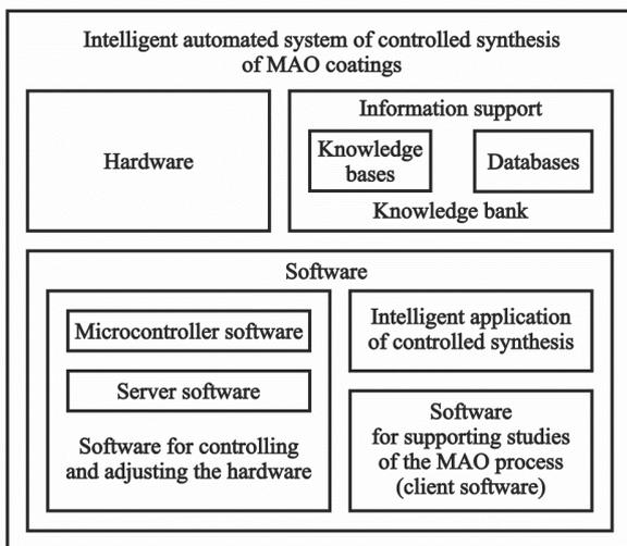
Fig. 1. The structure of the intelligent automated system of controlled synthesis
