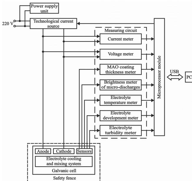
Fig. 4. The hardware structure of the intelligent system
