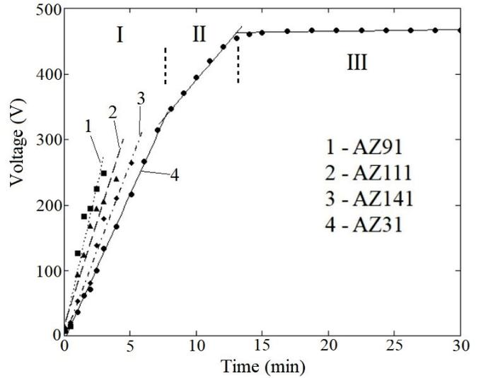
Fig. 8. Slope of forming curves at the anodizing stage (area I) for different magnesium alloys
