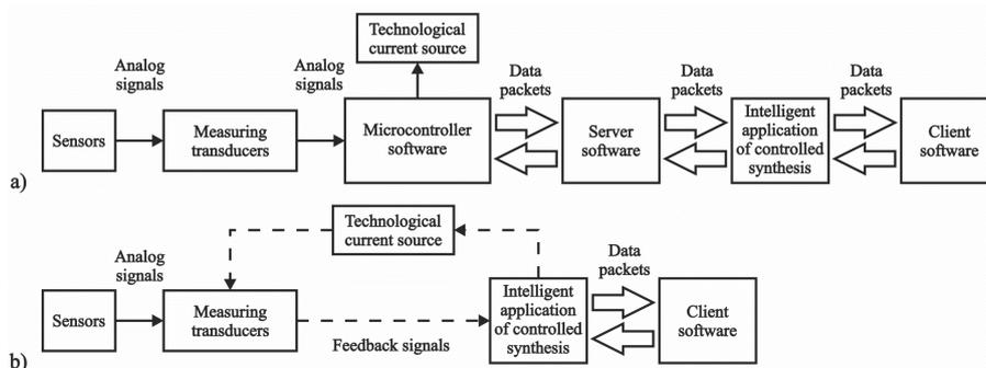
Fig. 6. The model of hardware and software interaction of the intelligent system: a) actual, b) with the feedback
