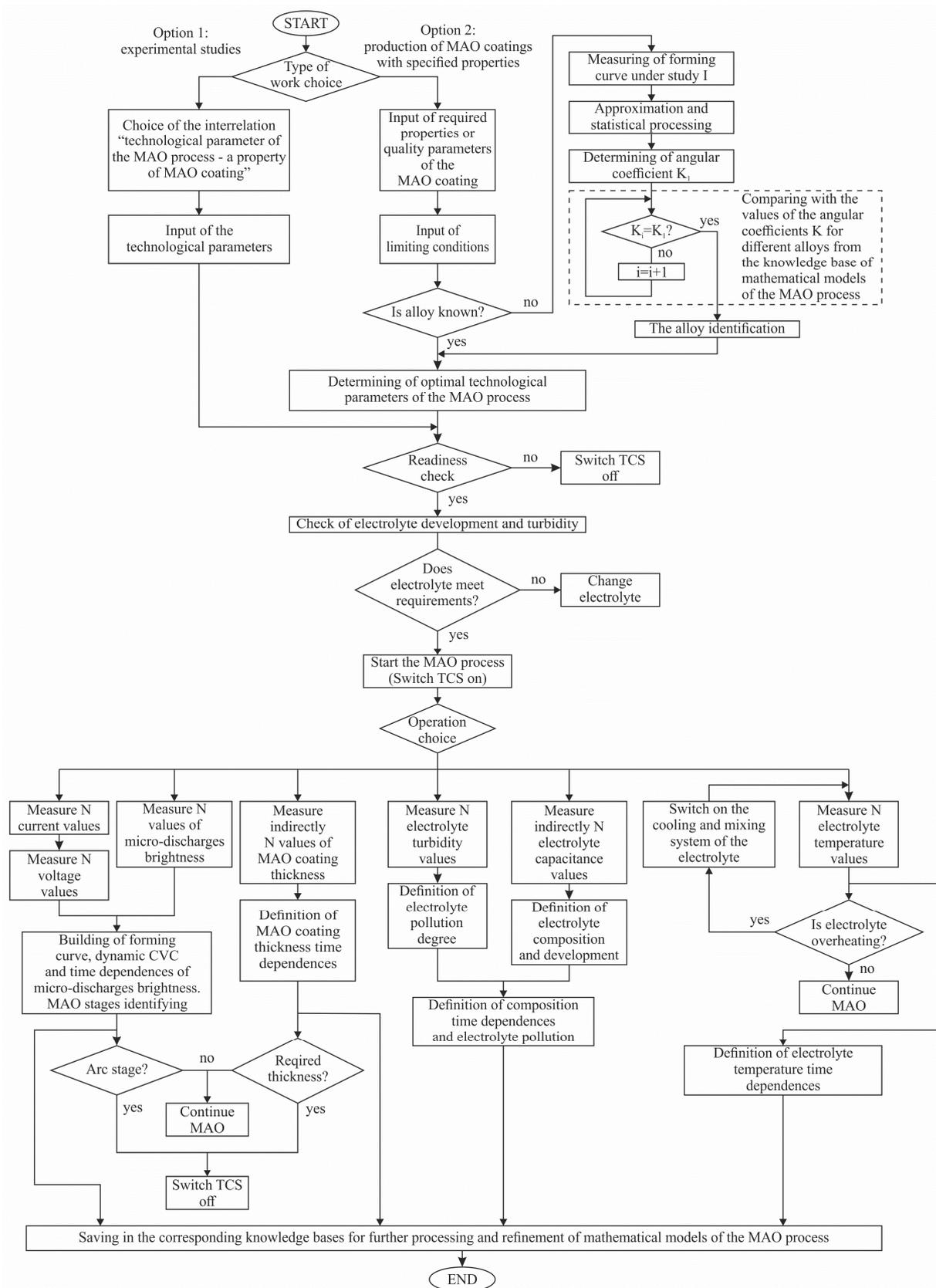
Fig. 7. Algorithm of the intelligent system software functioning
