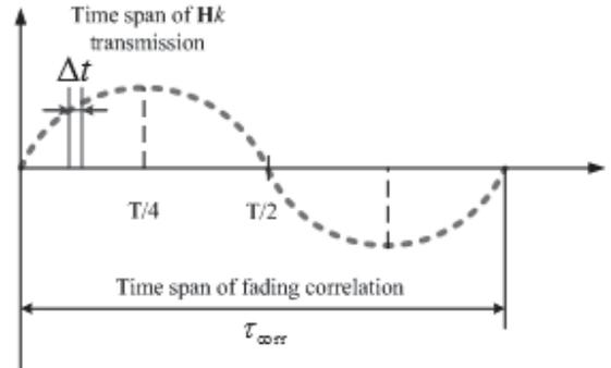
Fig. 6. Time span of channel matrix transmission
