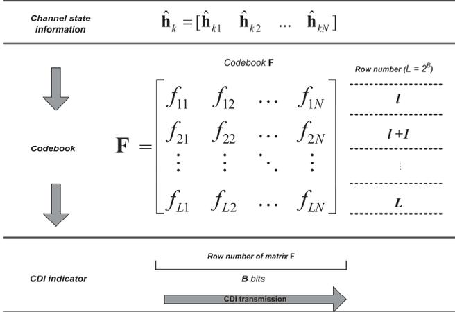
Fig. 5. Process of channel matrix quantization using first approach
