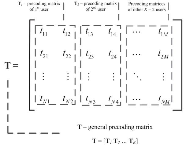
Fig. 3. Structure of general BS's precoding matrix
