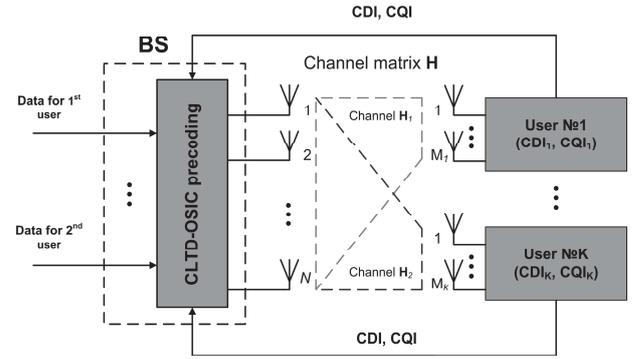
Fig. 2. MU-MIMO system with limited feedback
