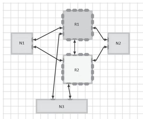
Fig. 12. SpaceWire network topology for the simulation
