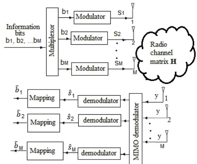
Fig. 1. MIMO system block diagram
