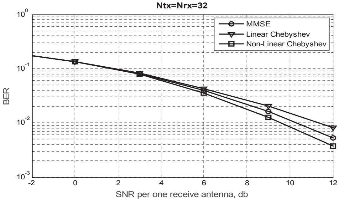
Fig. 3. BER performance of MMSE demodulation algorithm and linear and nonlinear Chebyshev iterative demodulation algorithms for the case of 32 transmitting and 32 receiving antennas
