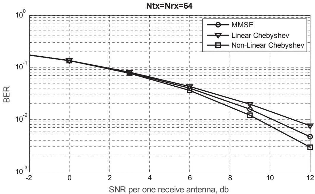
Fig. 4. BER performance of MMSE demodulation algorithm and linear and nonlinear Chebyshev iterative demodulation algorithms for the case of 64 transmitting and 64 receiving antennas
