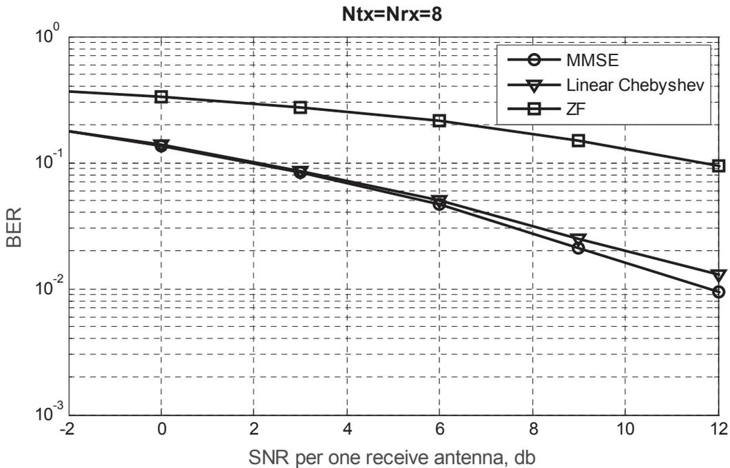
Fig. 2. BER performance for ZF and MMSE demodulation algorithms and Chebyshev linear iterative demodulation algorithm for the case of 8 transmitting and 8 receiving antennas
