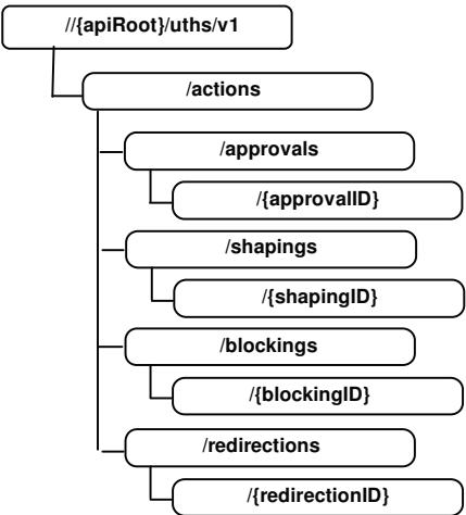
Fig.3 Structure of resources supported by UTHS
