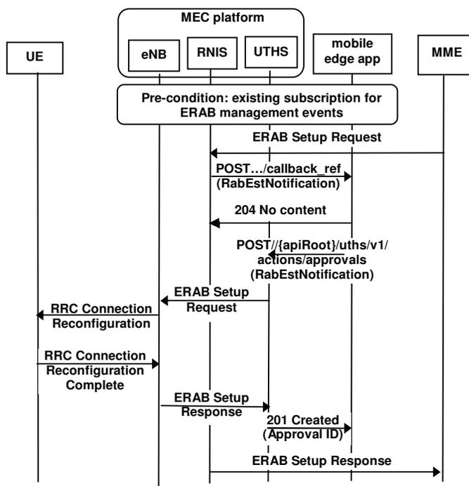
Fig.1. An approval of ERAB setup request by an authorized mobile edge application
