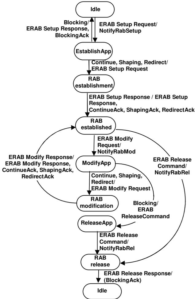
Fig.5. ERAB state model supported by MEC platform
