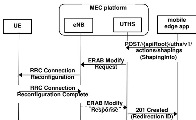
Fig.2. User traffic shaping by an authorized mobile edge application
