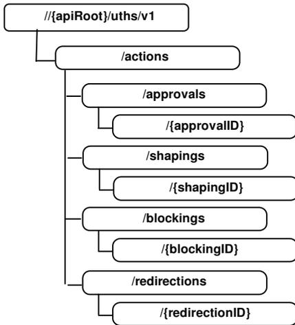
Fig.3 Structure of resources supported by UTHS
