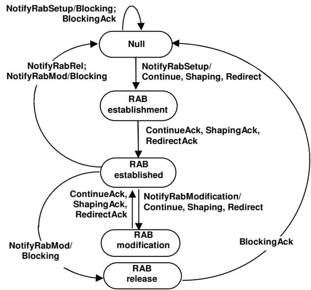
Fig.4. ERAB state model supported by a mobile edge application
