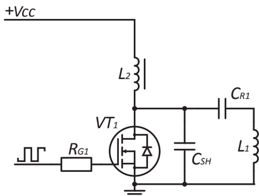
Fig. 4. Diagram of a power amplifier operating in key mode (class E)
