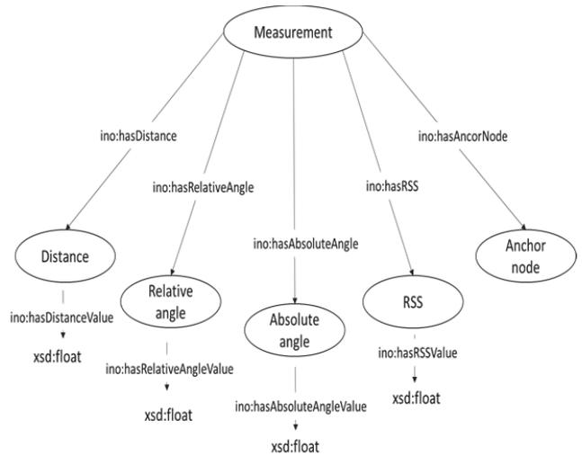
Fig. 5. Indoor Navigation Ontology fragment related to Measurement concept
