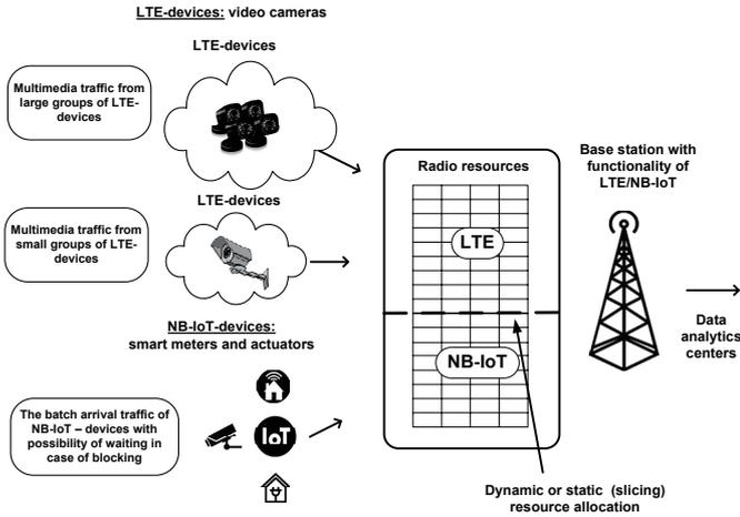
Fig. 1. The model of sessions forming by LTE and of NB-IoT devices
