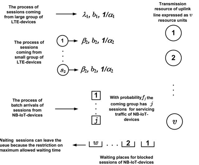
Fig. 2. The model of conjoint servicing of real time and batched NB-IoT traffic streams over LTE cell
