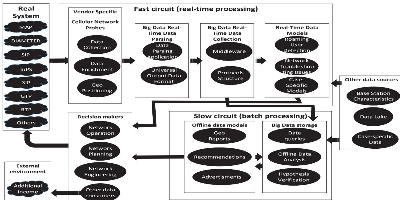
Fig. 1. The architectural overview of the DBDF – a concept
