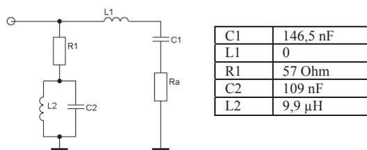
Fig. 4. Circuit configuration and ratings of the frequency-extension circuit elements
