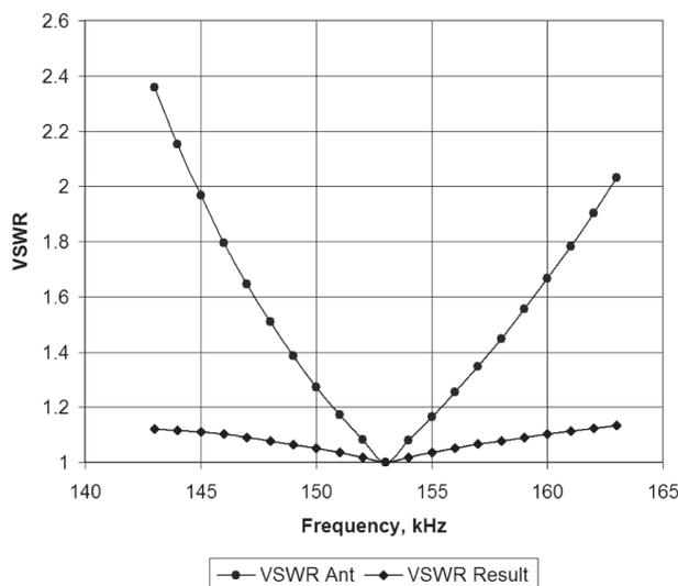
Fig. 5. The initial antenna VSWR and the resulting antenna VSWR with a frequency-extension circuit
