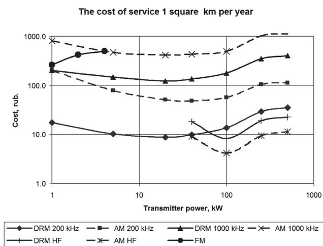
Fig. 1. The cost of servicing one square kilometer of territory per year (rubles, excluding VAT) by transmitters of various power and frequency ranges
