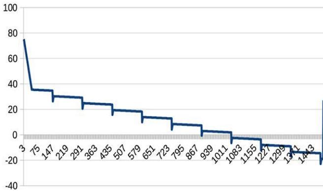
Fig. 14. Difference in the amount of service information in 1 channel with packets of up to 1500 bytes
