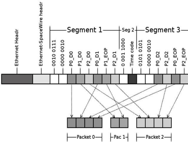
Fig. 9. Transmission of three packets and one Time Code
