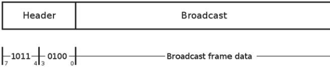
Fig. 7. Broadcast segment structure
