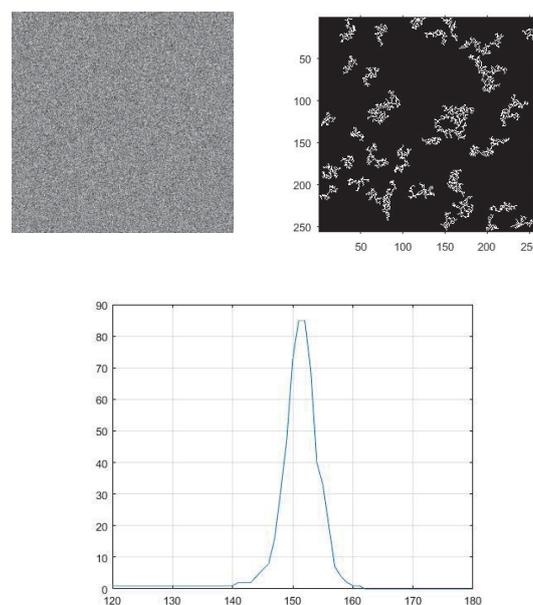
Fig. 2. Noise binarization and the dependence of false objects number from threshold value
