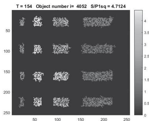
Fig. 8. Selection of objects on the test image by the elongation coefficient of the main axes. The inverse value was calculated.
