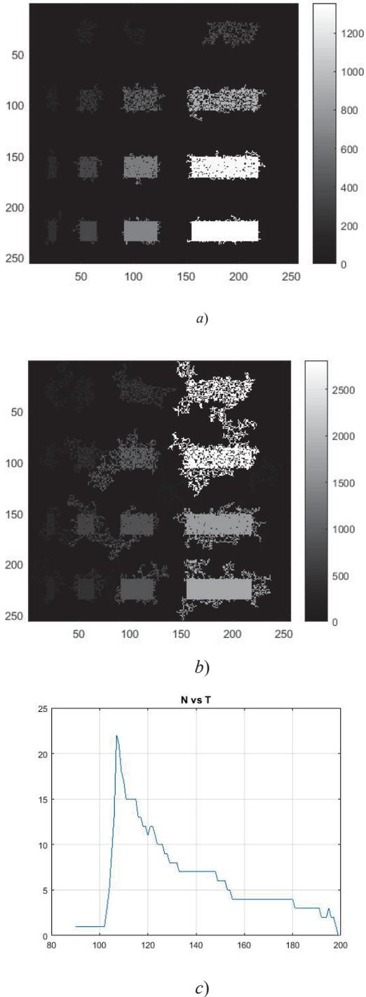
Fig. 3 The result of single-threshold selection of rectangular objects and the dependence of the number of selected objects on the threshold value: a)  $T=115$ ; b)  $T=108$ . The brightness of objects is proportional to their area
