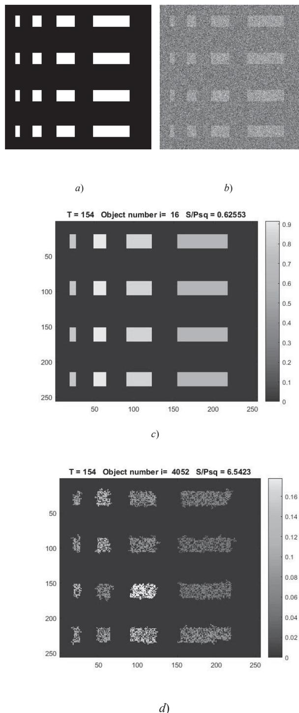
Fig. 6. Selection of objects on the test image by the ratio of elongation of the perimeter. The inverse value of  $1/P_S$ , which corresponds to the scale on the right, was calculated.
