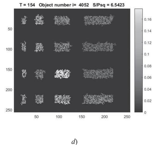
Fig. 6. Selection of objects on the test image by the ratio of elongation of the perimeter. The inverse value of  $1/P_S$ , which corresponds to the scale on the right, was calculated.
