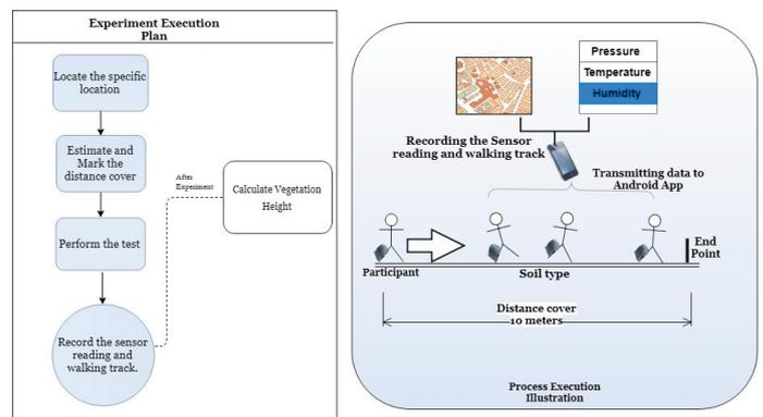
Fig. 4. General execution plan of the experiment setup
