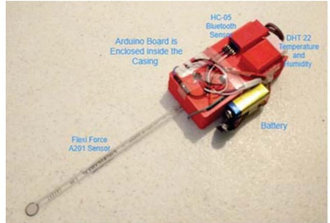
Fig. 2. Wearable platform representation: image view of the developed system
