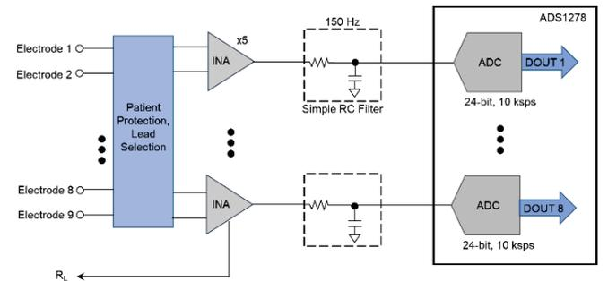
Fig. 3. Structure of a Sigma-Delta ADC based cardiograph
