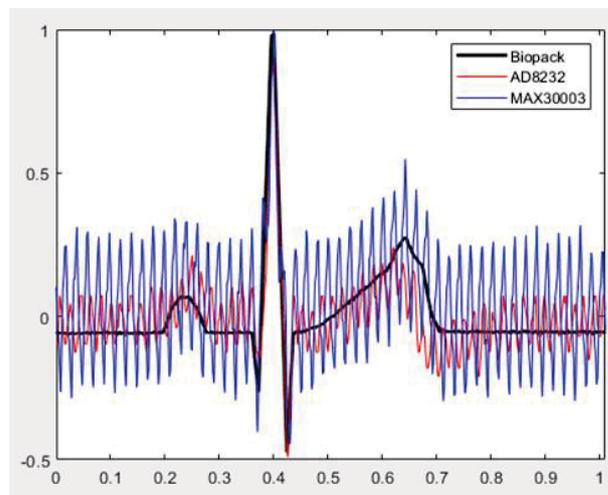
Fig. 4. “RAW” signals from different sources
