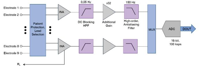
Fig. 2. Structure of a standard SAR-based cardiograph
