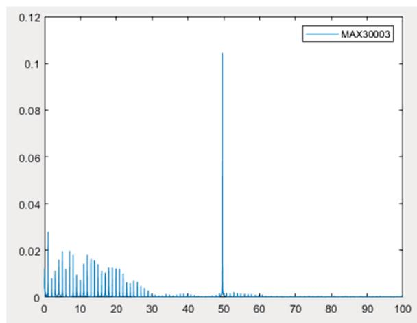
Fig. 5. Fourier transformation of MAX30003 signal
