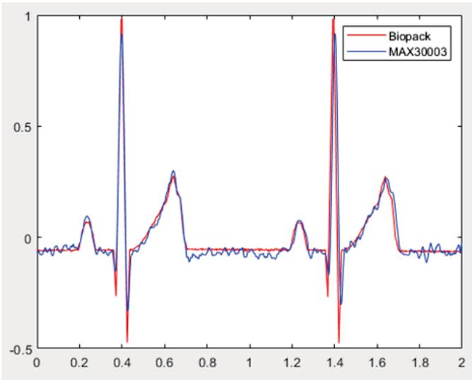
Fig. 6. Digitally filtered MAX30003 signal.
