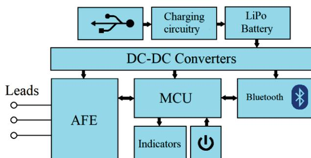
Fig. 1. Structural scheme of a portable cardiograph
