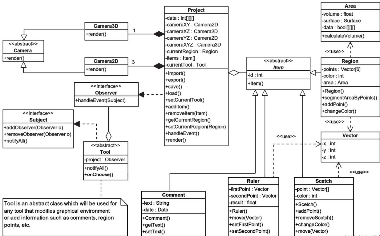
Fig. 2. Class diagram of the service
