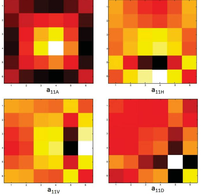
Fig. 1. Block structure of basis image for wavelet  $db6$ . There are four  $6 \times 6$  matrices  $a_{11A}$ ,  $a_{11H}$ ,  $a_{11V}$  and  $a_{11D}$ . They belong to blocks that refer to approximation coefficients, horizontal, vertical and diagonal details
