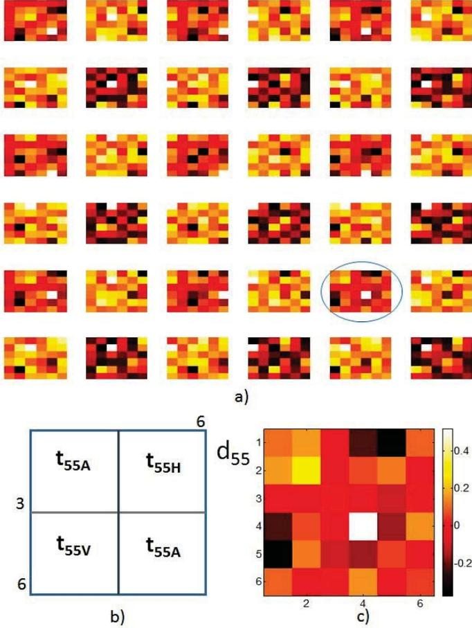
Fig. 2. Block structure of basis images  $d_{kp}$  for wavelet  $db6$ ,  $N = 6$ . a) The set of 36 items, every item has block structure. b) and c) Four blocks of coefficients of image  $d_{55}$
