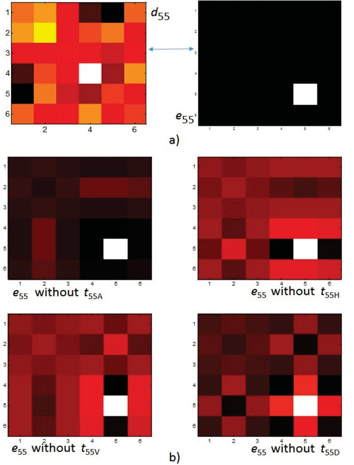
Fig. 3. Properties of the coefficient blocks for basis image. a) Image  $d_{55}$  is transformed from original image  $e_{55}$ . b) The retrieved original after removing from  $d_{55}$  one of the blocks: approximation coefficients, horizontal, vertical and diagonal details
