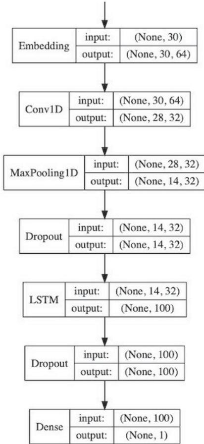
Fig. 1. CNN + LSTM neural network architecture
