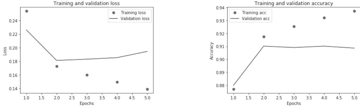
Fig. 3. Training of CNN + LSTM model. Comparing results on training and validation sets from Rubtsova’s corpus
