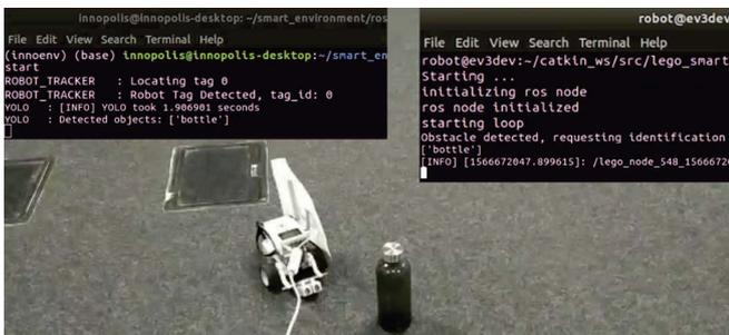
Fig. 9. Smart Space’s node identifies the robot location and obstacles around the robot, and sends the list of obstacles detected back to the robot
