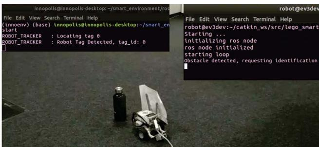
Fig. 8. As the robot detects an obstacle, it stops and publishes a message to request the Smart Space’s node to identify obstacle
