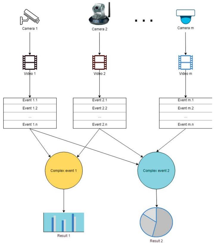
Fig. 3. Event model Based on Video Streams
