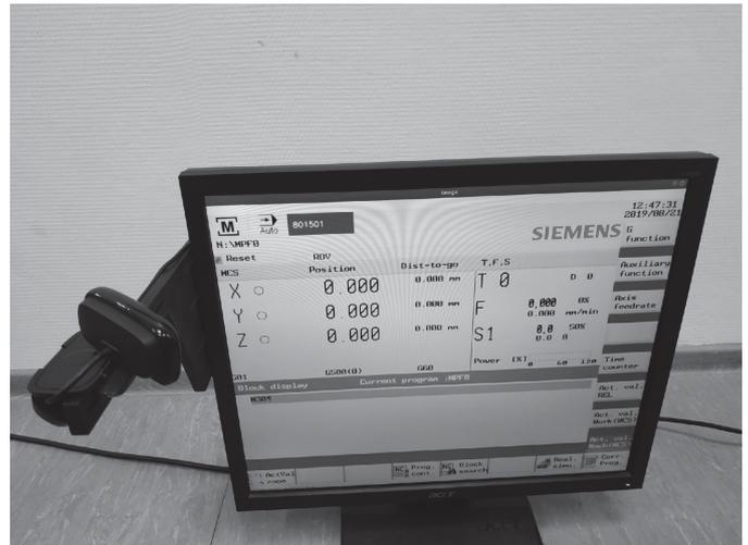
Fig. 5. Machine stand emulator: front view
