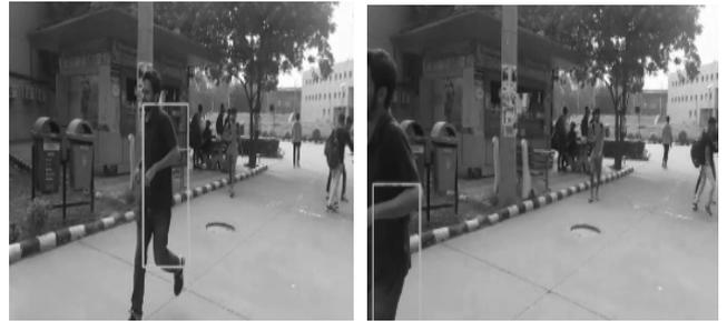
Fig. 8. A person running classified as an anomaly and being tracked by the camera C1.
