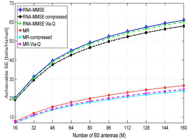
Fig. 1. Achievable SE per RRH vs. number of RRH antennas with a reuse factor of 1
