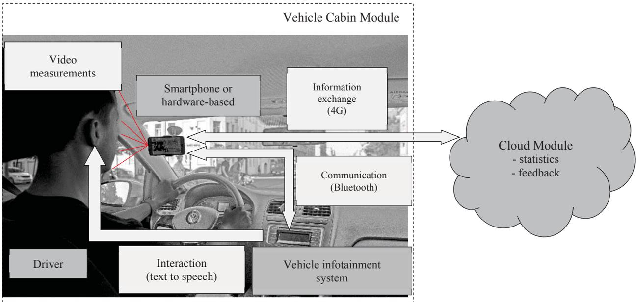
Fig. 2. Driver monitoring system
