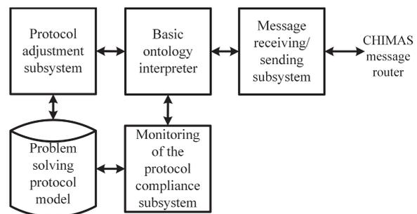
Fig. 6. The architecture of the protocol control agent
