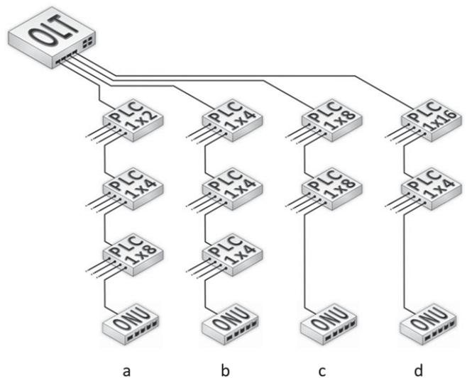
Fig. 1. Typical examples of PON topology
