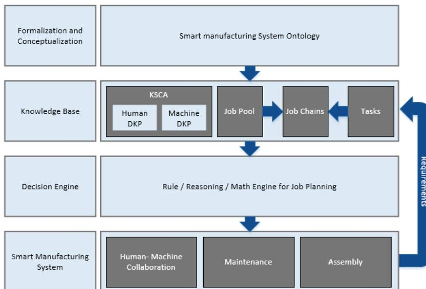
Fig. 3. Research framework of ontology-based planning in smart manufacturing systems
