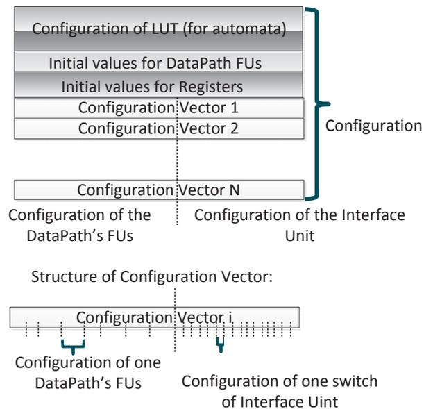
Fig. 4. Structure of configuration
