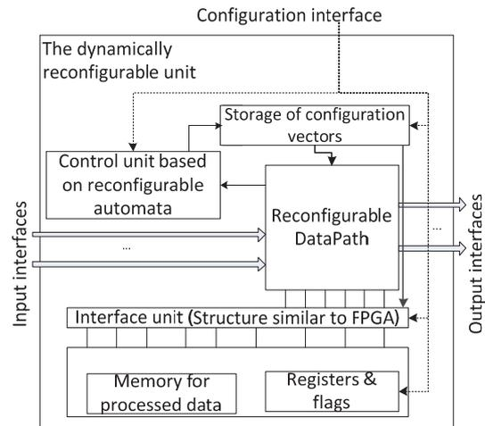
Fig. 3. General structure of the proposed dynamically reconfigurable unit
