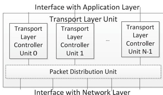
Fig. 1. Typical structure of transport layer unit
