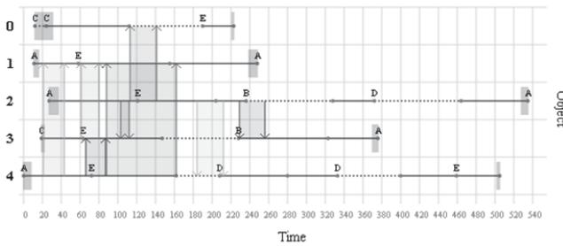
Fig. 8. An example of a visualization of the schedule for moving objects (objects are arranged vertically, the horizontal axis corresponds to the observation time). The horizontal lines correspond to the movement of the object between the control nodes. Vertical arrows visualize meetings and possible transmissions between objects.
