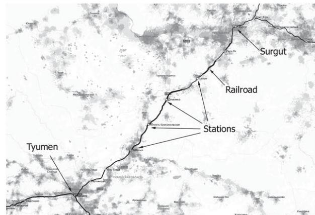
Fig. 13. Tyumen-Surgut railroad coverage map (for one mobile network carrier, MTS). Color intensity corresponds to quality of coverage.
