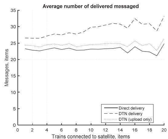
Fig. 21. Average number of delivered messages per train (only for the trains that are not connected to a satellite) depending on number of trains connected to satellites
