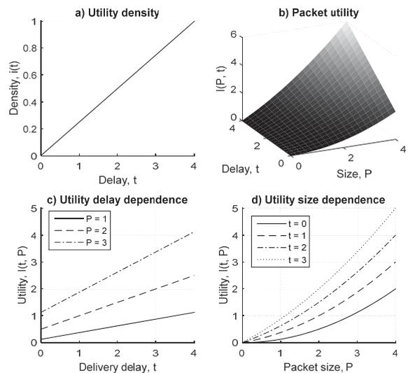
Fig. 4. Average delay (linear utility) estimation of the packet depending on the packet duration  $P$  and the transmission packet delay  $t$  (for  $t_0 = 4$ )
