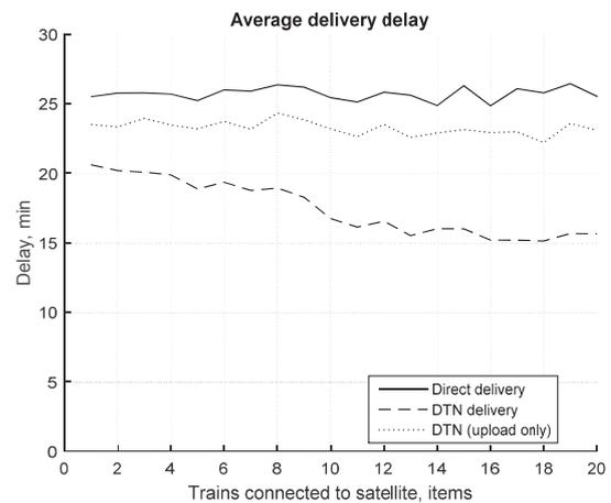
Fig. 22. Average delivery delay (only for the trains that are not connected to a satellite) depending on number of trains connected to satellites.
