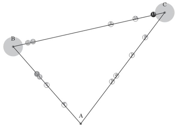
Fig. 7. An example of visualization of nodes location (denoted by letters), their connections, BS at some nodes (coverage is marked with big light gray circles around the nodes), objects (indicated by numbers) and TS coverage (small circles: normally without filling, gray while meeting TS, dark gray if connected to BS) at some time.
