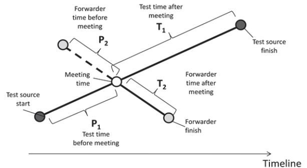
Fig. 5. Estimation model visualization: “test” object (data generating source) is moving from start to finish during the time  $P_1 + T_1$ , and in time  $P_2 + T_2$  after the start meets the “forwarder”, who will finish earlier, in time  $T_2 < T_1$
