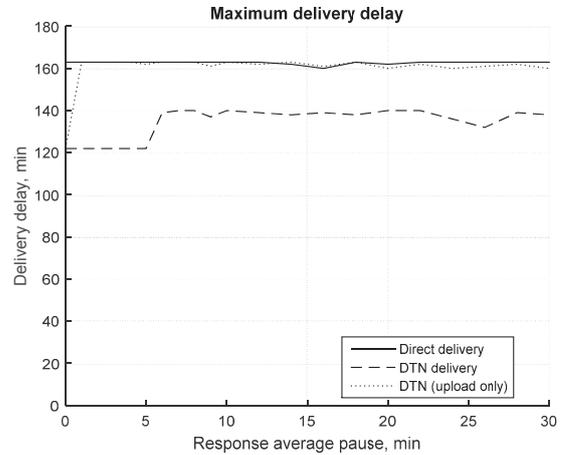
Fig. 17. Maximum delivery time with response-to-request message scheme depending on average response time (normally distributed random value) for all mobile operators available.
