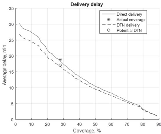
Fig. 19. Average delivery delay depending on coverage area (scaled from existing now)
