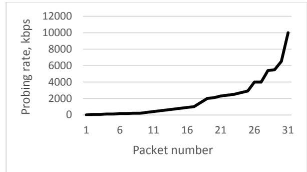
Fig. 5. Relationship between instantaneous probing rate and probing packets order,  $N = 30$  packets,  $\Delta T = 0.5$  ms,  $\Delta P = 50$  bytes
