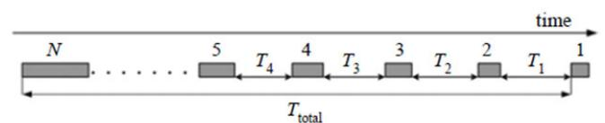
Fig. 4. Probing train of  $N$  packets
