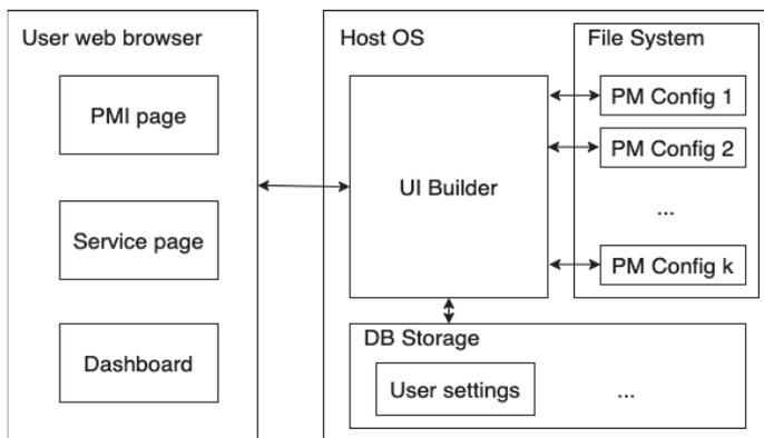
Fig. 4. System User Interface architecture
