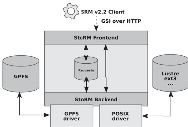
Fig. 1. Abstract of the StoRM components and the relationship between FE and BE components. The client request is taken through the FE interface, who decides, according to its type, to process or forward it to BE module. The memory access is done through the BE component using the access drivers to the distributed file system composed by different technologies [11].
