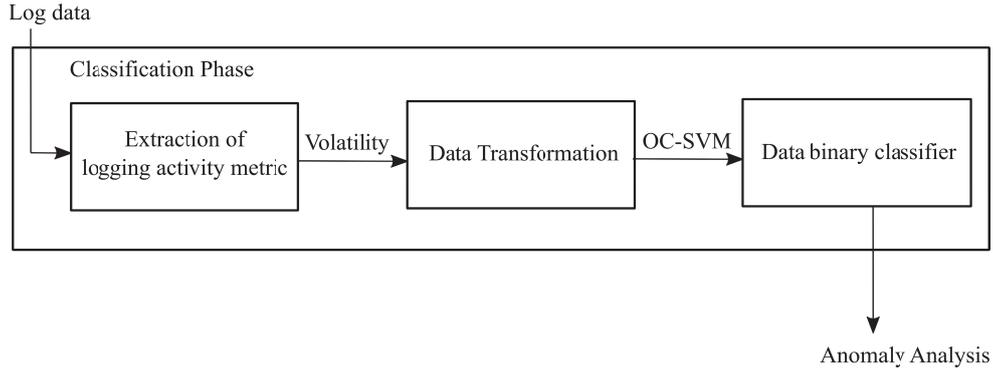
Fig. 3. Data flow diagram of the proposed diagnostic system, highlighting the main steps of the solution, from the raw log data input to the anomaly classification as output.
