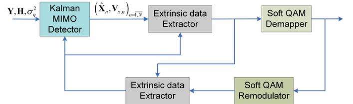
Fig. 3. Block diagram of an iterative receiver for a system with a MIMO channel and distributed spatial multiplexing
