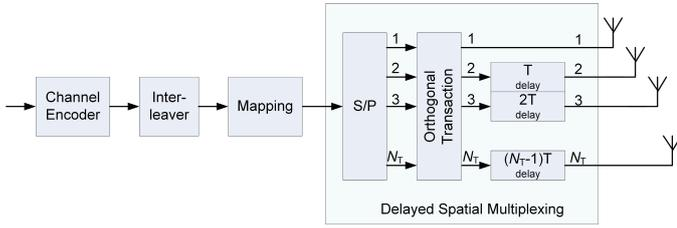
Fig. 2. Block diagram of the transmitting part of the system with a MIMO channel and distributed spatial multiplexing
