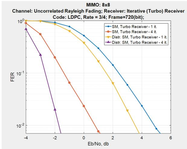
Fig. 4. FER versus signal-to-noise ratio per bit for a MIMO system with conventional spatial multiplexing and distributed spatial multiplexing
