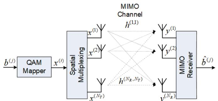
Fig. 1. System model of MIMO set-up with spatial multiplexing
