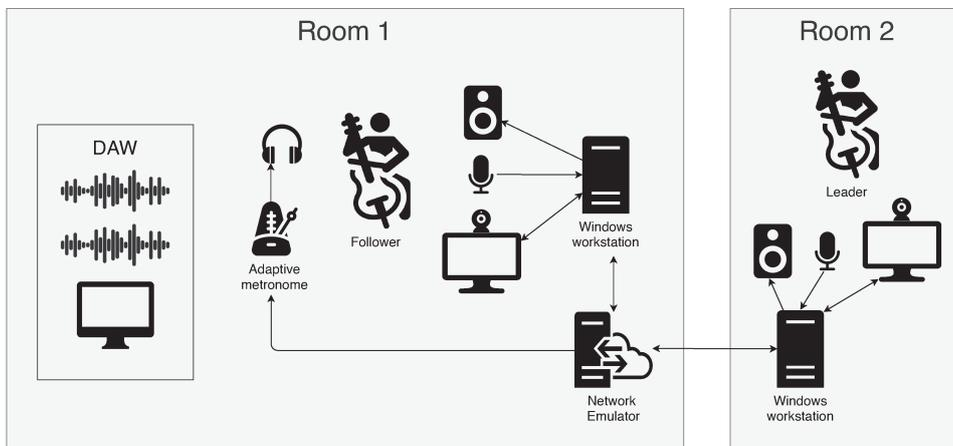
Fig. 3. Setup of the experiment
