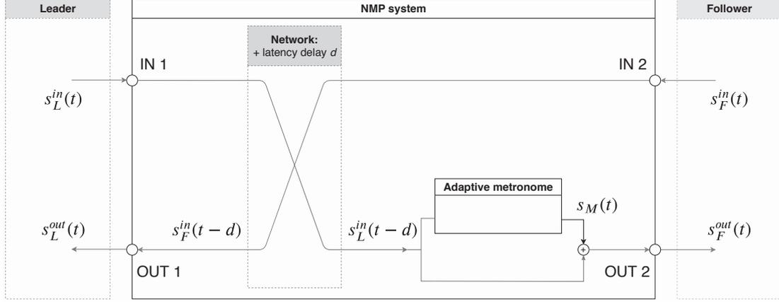
Fig. 1. Schematic representation of the adaptive metronome technique
