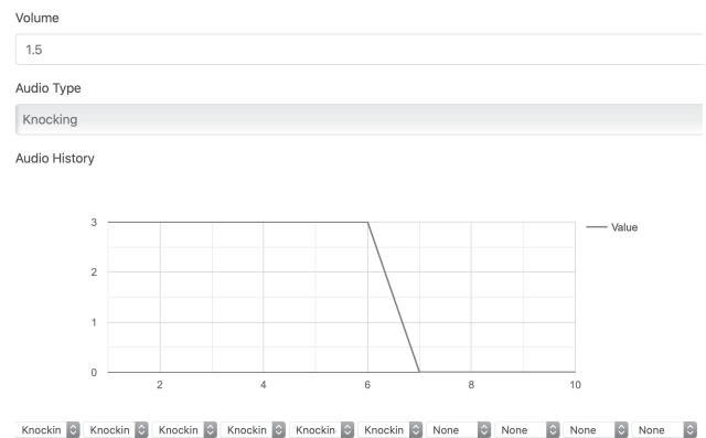
Fig. 4. Volume and Audio Type shows the current state of machinery. Audio History provides information when the failure has started and the type of audio failure. Y-axis represents the type of audio the X-axis the hours.
