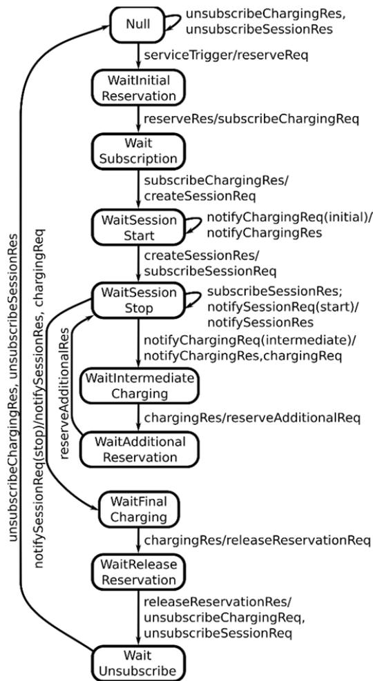
Fig.3 Charging state model, supported by a mobile edge charging application
