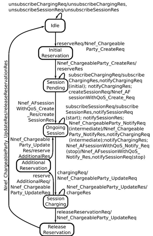
Fig.4 Charging state model, supported by a mobile edge platform
