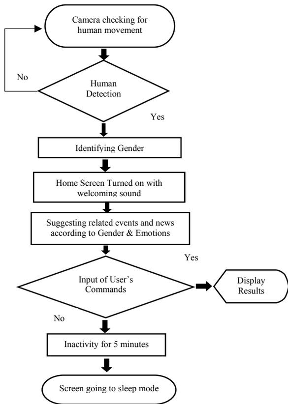
Fig. 2. Image Processing Flowchart
