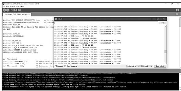
Fig. 13. Resultant data from the sensors (Temperature, Humidity, RFID – Denied Access) observed in the serial monitor
