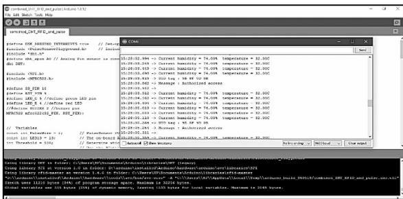
Fig. 12. Resultant data from the sensors (Temperature, Humidity, RFID - Granted Access) observed in the serial monitor
