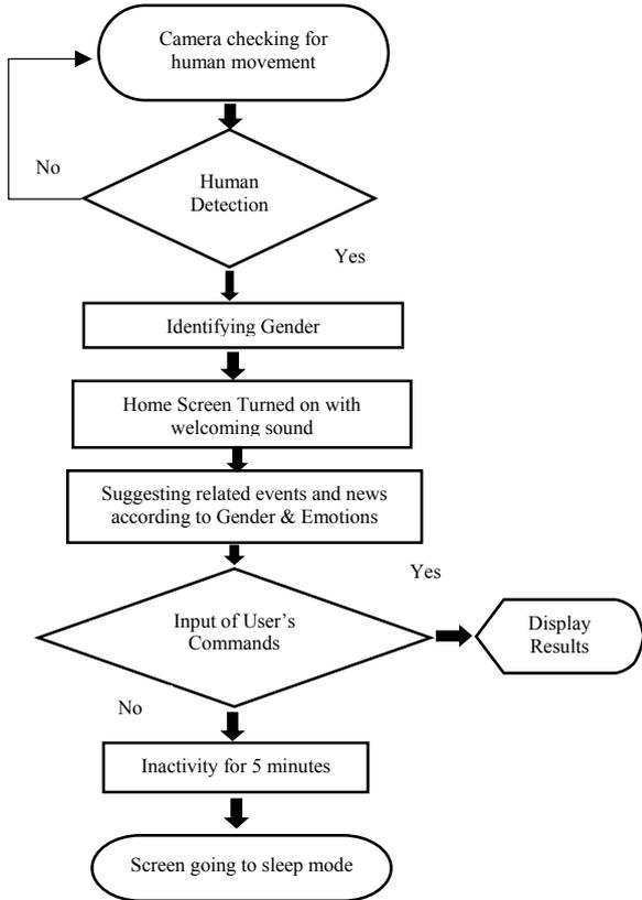
Fig. 2. Image Processing Flowchart
