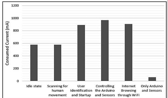
Fig. 15. The current consumption rate of various tasks & states
