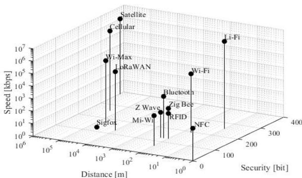
Fig. 4. Signal processing speed, communication nodes distance and communication channel security
