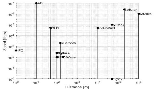
Fig. 1. Signal processing speed and communication nodes distance
