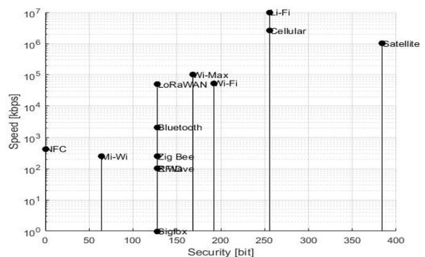
Fig. 2. Signal processing speed and communication channel security
