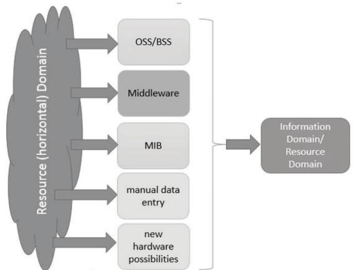
Fig. 4. Source systems for the Resource Horizontal Domain
