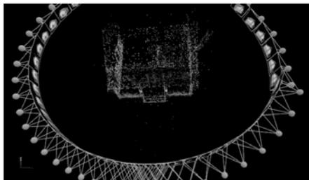
Fig. 6 Arrangement of cameras. Points are the cameras' position in space; the corresponding rectangle is the image in the camera lens
