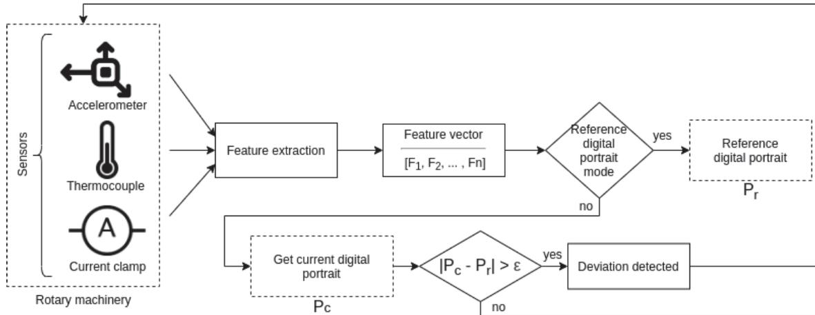
Fig. 1. Data flow for a deviation detection model based on a feature vector
