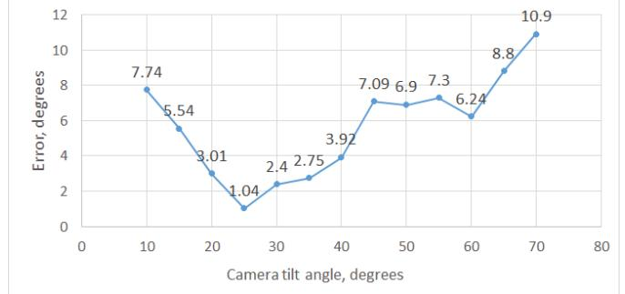
Fig. 9. A graph of the ground plane normal estimation error versus the camera tilt angle
