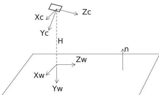
Fig. 3. An example of placing a surveillance camera relative to the ground plane
