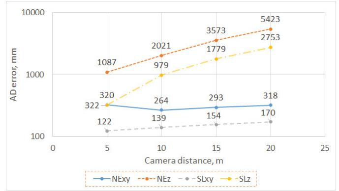
Fig. 5. AD error graphs versus the camera distance
