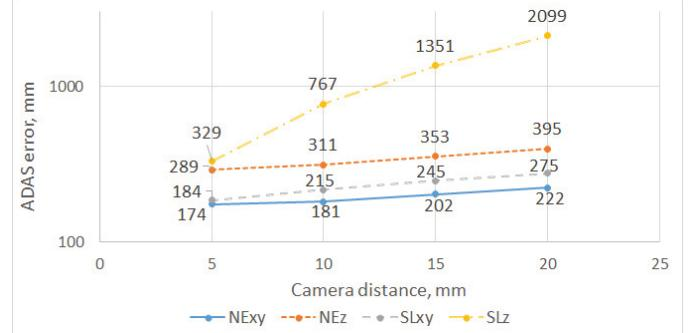
Fig. 6. ADAS error graphs versus the camera distance
