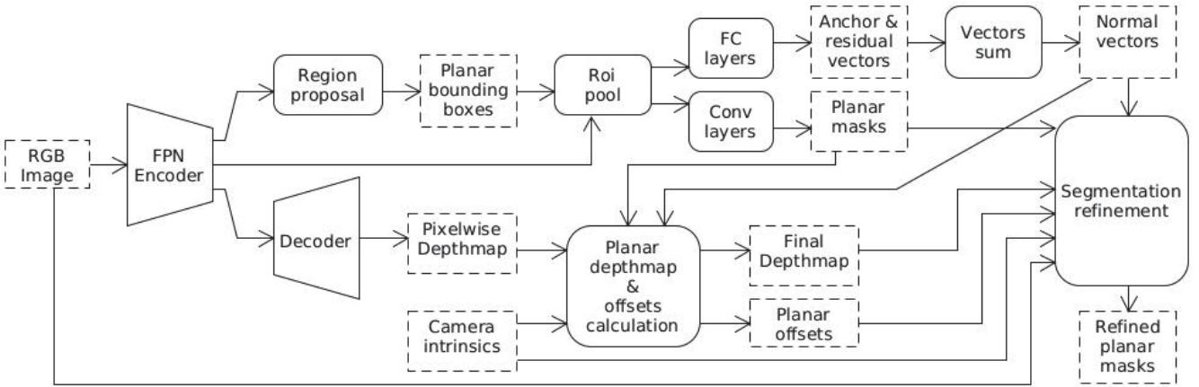
Fig. 2. A diagram of the PlaneRCNN neural network for detecting planes in images
