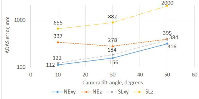
Fig. 8. ADAS error graphs versus the camera tilt angle
