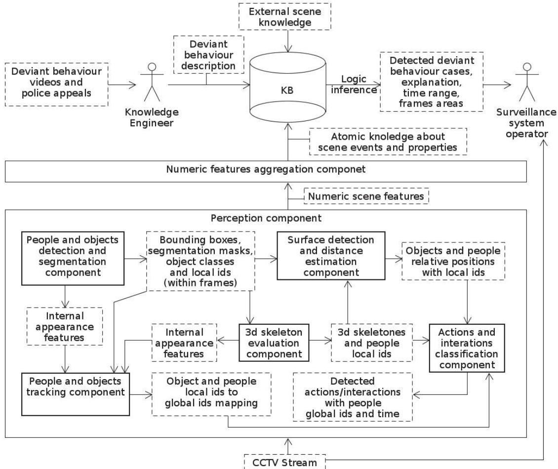
Fig. 1. Diagram of the approach for detecting deviant behavior of people via city surveillance cameras
