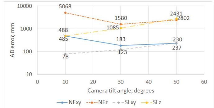
Fig. 7. AD error graphs versus the camera tilt angle
