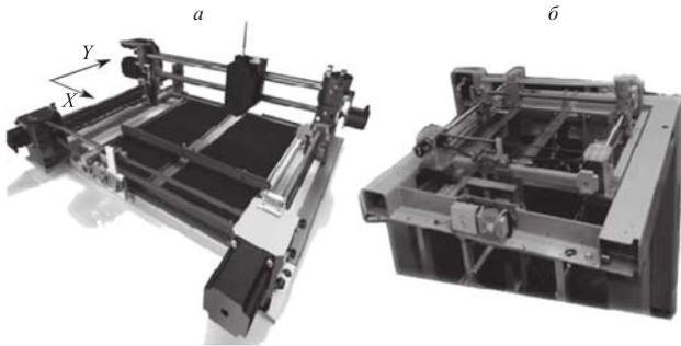
Fig. 5. Platform in Solidworks (a) and assembled (b) [24]
