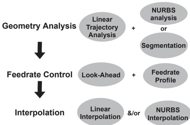
Fig. 3. The structure of developed trajectory planner
