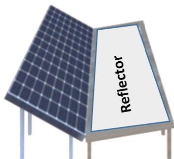
Fig.5 Proposed fixing of the reflectors
