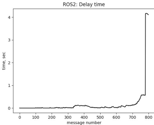
Fig. 6. ROS2's delay time with 200 msgs/sec
