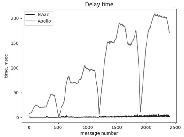
Fig. 13. Isaac, Apollo delay time with 1000 message per second frequency
