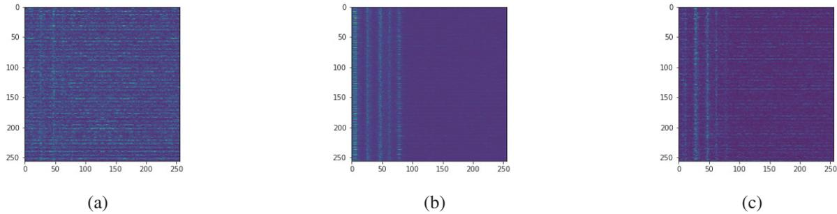
Fig. 1. The spectrogram examples: healthy (a), outer race defect (b), and inner race defect (c)
