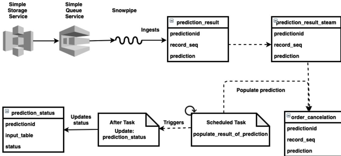
Fig. 5. Flow diagram of piping the data into Snowflake
