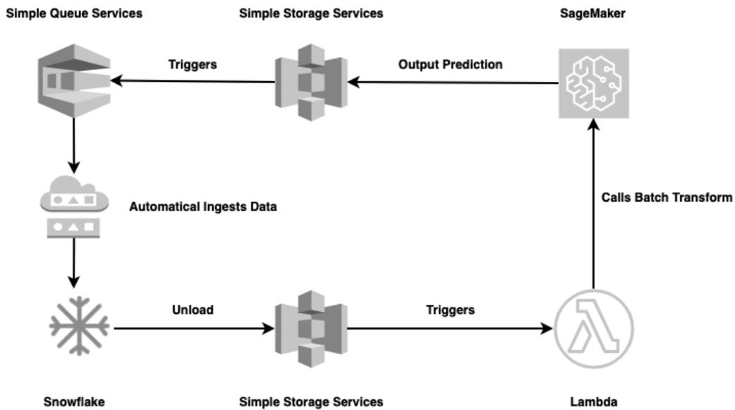
Fig. 1. Diagram of proposed architecture
