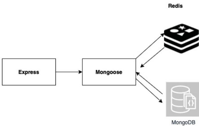
Fig. 4. Design schema of the proposed database module
