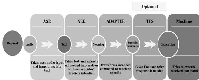
Fig. 5. Pipeline of proposed integration from request to execution
