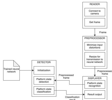
Fig. 12. Computer vision software module structure
